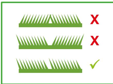
**Step 1** Adjacent rolls should be laid together with the grass pile pointing in the same direction.
