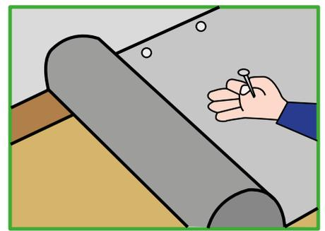
**Step 3** Lay your weed barrier over the sand, pegging the weed barrier to the wooden battens when possible to help hold it in place.
