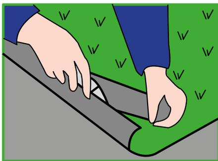
**Step 4** Step 4 Using a sharp Stanley knife; carefully cut around obstacles and cut away any excess artificial grass material that isn't required.
