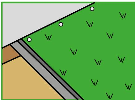
**Step 5** Using wood/decking screws fix your new artificial lawn directly over and onto the wood battens. Trimming any excess grass off using a sharp Stanley knife.
