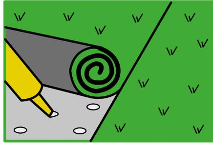
**Step 2** Rolls can be loose laid or fixed with a spots of outdoor adhesive or with double-sided adhesive tape.
