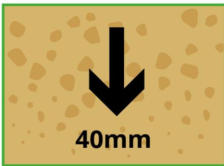
**Step 1** Remove your top layer of turf and continue digging down to 40mm depth. Flatten the earth down. Wooden timber battens can be installed around the perimeter to allow you to screw and secure your artificial grass into place.
