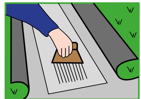
**Step 3** Apply the adhesive to the top surface of the seaming tape. Fold artificial grass edges onto the joining tape and glue. Use weight on top of the artificial grass over night to enhance the strength of the joint.
